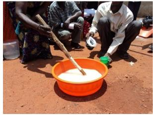
Sodium Hydroxide solution preparation
