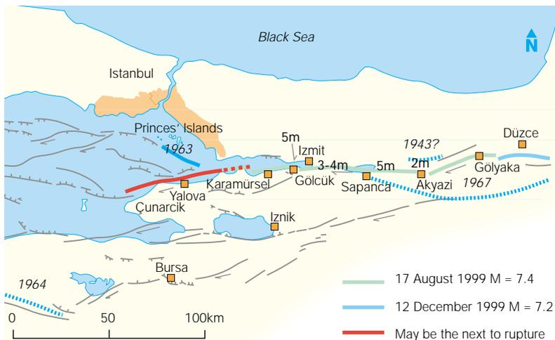
1. Location of Yalova, showing recent and postulated fault ruptures. Dates are year in which fault segment ruptured.
