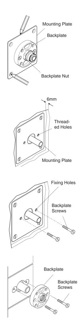
14. Fit the olive over the copper pipe and tighten the backplate nut into position.
