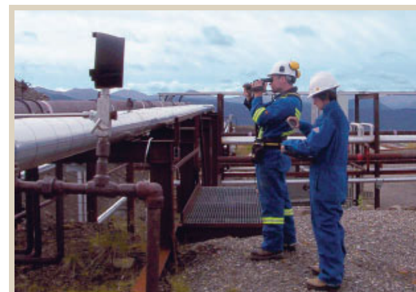
Roxanne Pettipas and Terence Trefiak survey pipelines in Canada with an infrared camera.
