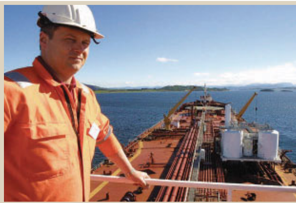
The Randgrid master on the bridge, overlooking the white VOC recovery unit.
