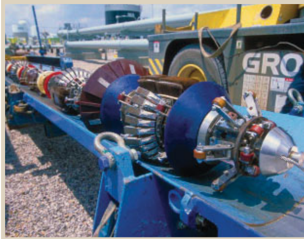
Smart pigs, like the one pictured above, can precisely locate internal or external defects, such as cracks, dents or corrosion.
